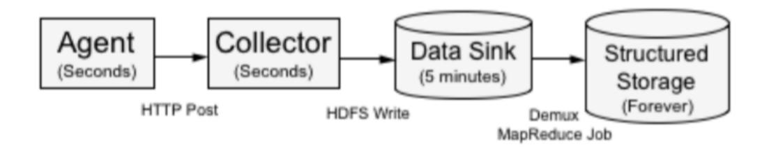
Figure 1: The Chukwa Pipeline, showing how long data is retained at each stage.
